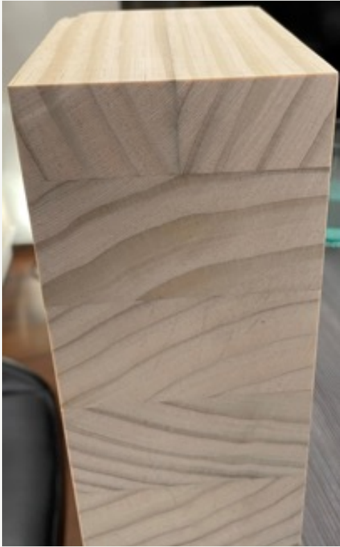
Top lamela from glulam showing vertical grain. Endgrain must be protected.
