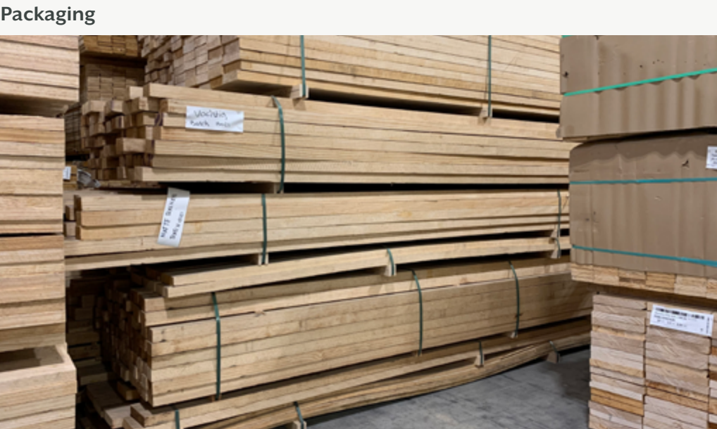
Bundles stored on top of each other; bearers aligned
