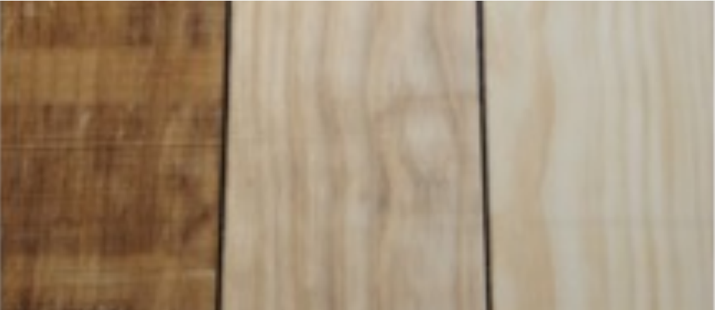
Discolouration of rough board, after surfacing 3mm / 0.12" and after surfacing 6mm / 0.24" from rough
